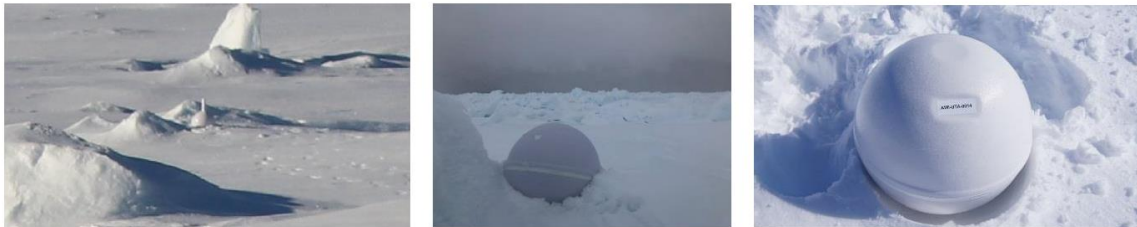
Fig. 2: drifter buoys near the Larsen Ice Shelf were frozen in the Larsen B embayment. Buoys in the east capture the general flow characteristics in the central Weddell Sea.
