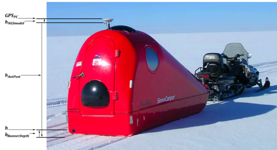
Figure 2. GPS antenna, sled, and snowmobile configuration.
