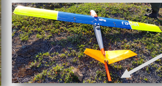
Fixed-wing with multispectral camera Parrot Sequoia.
