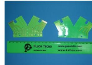
Printed Circuit Board (PCB)
