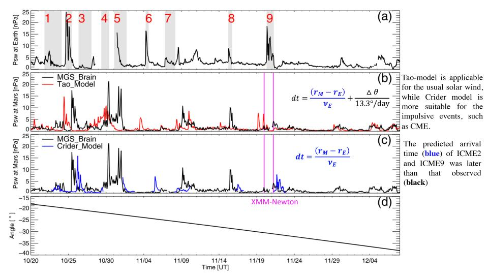
Panel (a): the P<sub>sw</sub> at Earth from OMNI. The light grey filled rectangles label the ICMEs at Earth identified by Jian et al. (2006). Dark curves in panels (b)–(c): the P<sub>sw</sub> estimated from the MGS observation ( $\sim \frac{B_{subsolar}^2}{2\mu_0}$ ). Red curves in panel (b) : the P<sub>sw</sub> predicted by the Tao model. Blue curves in panel (c) : the P<sub>sw</sub> predicted by the Crider model. Panel (d): the Earth–Sun–Mars angle.
