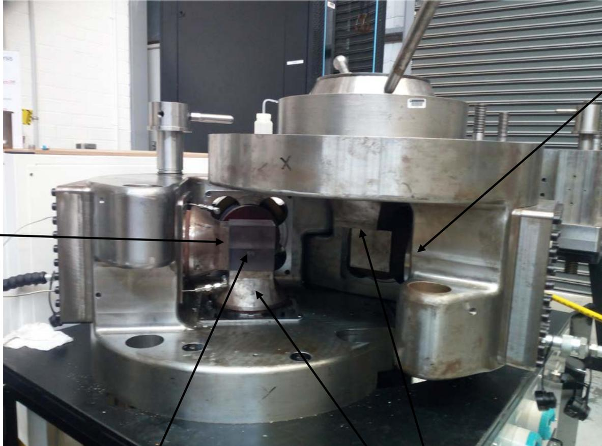
The loading platens applying  $\sigma_2$
