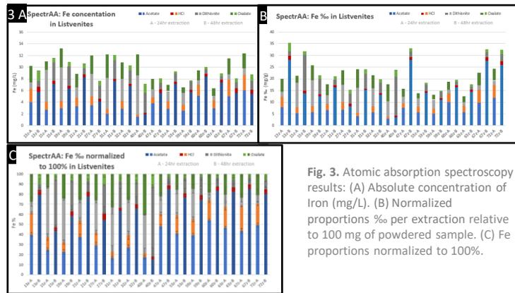
Fig. 3. SpectraAA: Fe concentration results: (A) Absolute concentration of iron (mg/L). (B) Normalized proportions % per extraction relative to 100 mg of powdered sample. (C) Fe proportions normalized to 100%.
