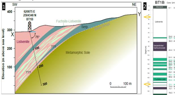
Fig. 1. Cross Section of BT1B<sup>2</sup> Fig. 2. Stratigraphic column of BT1B<sup>2</sup> relative to core samples by depth from the surface. Studies samples between orange triangles.
