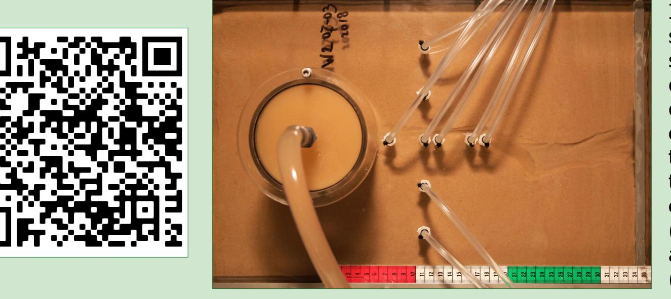
In a **laboratory setting**, several sand samples were mixed and subjected to a hydraulic head difference between an inflow filter on one side and a **single exit point** on the top of the experiment. As the top of the experiment was seethrough the **progress of the pipe** could be monitored visually (left). The results of this experiment are used to calibrate a digital model (right). See the QR code for an animated version
