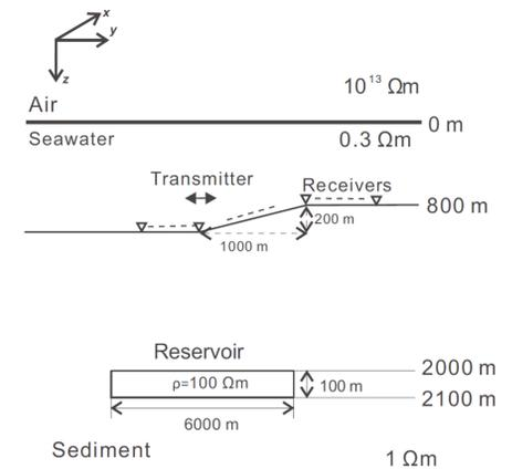
Fig. 3 The 1D reservoir model modified after Constable and Weiss (2006).
