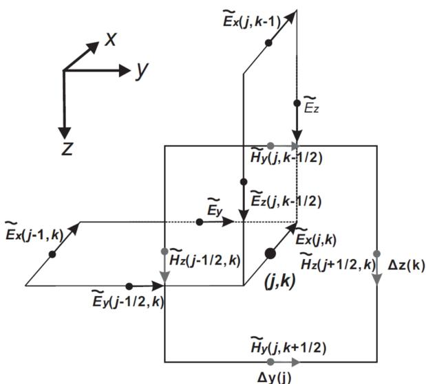
Fig. 1 The 2D staggered-grid for cell  $(j,k)$  modified after Li and Han (2017), where  $\Delta y$  and  $\Delta z$  are the horizontal size and vertical size, respectively.
