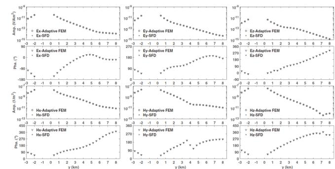
Fig. 4 Comparison of the 2.5D numerical results of the total fields for the 2D marine slope model shown in Fig. 3. The adaptive FEM results (denoted by circles for the electric components and triangles for the magnetic components, respectively) computed by MARE2DEM following Key (2016) are used for benchmarking the SFD results (denoted by crosses).
