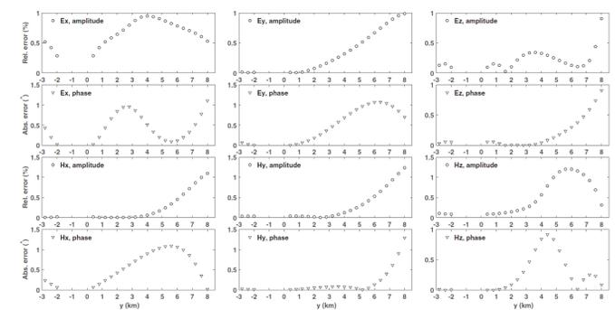
Fig. 5 The relative error of amplitudes (Rel. error, denoted by the circles) and the absolute error of phases (Abs. error, denoted by the triangles) for the 2.5D total field results benchmarked by the adaptive FEM results for the 2D marine slope model shown in Fig. 3.
