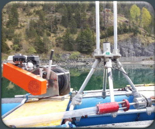
Piston Corer with Hammer Action Ø 63 mm
