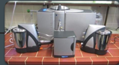
MALVERN Mastersizer 3000 Grain Size
