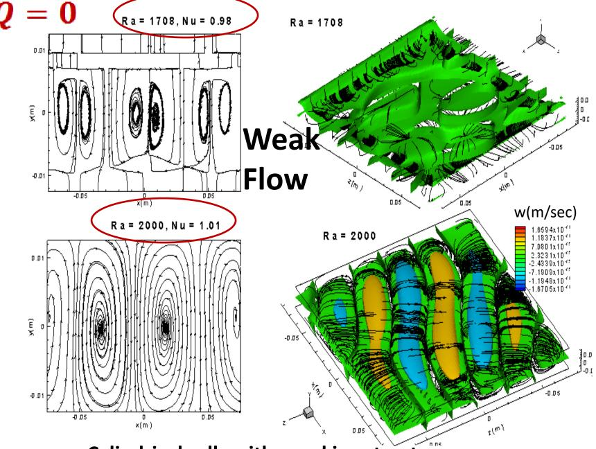
Cylindrical rolls with sneaking structures
