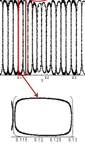
For Ra > 1708 we get symmetric rolls having y-axis as a axis of rotation.
