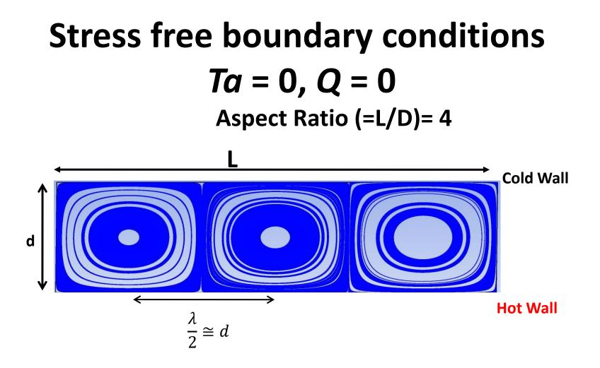
Diameter of the convection cells is half the critical wave-length  $\lambda_c = \frac{2\pi}{k_c} = 2.82$ ,  $k_c$  is the critical wavenumber and  $k_c = \pi/\sqrt{2}$ .
