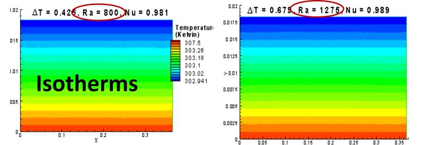
When Ra < 1708 we get Nu < 1, i.e., subcritical flow. Heat propagates in the system as a conduction mode.
