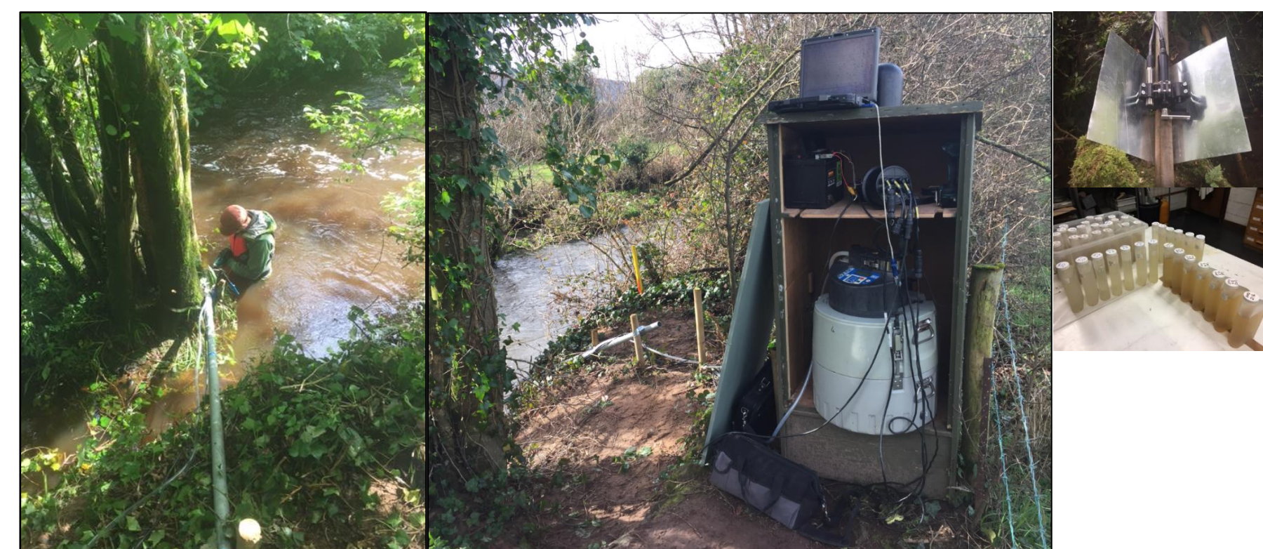
Fig. 3 Monitoring stations at each site are instrumented with auto-samplers, turbidity probes and water-level recorders.
