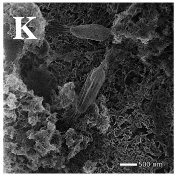
He Ion microscopy images of PE exposed to surface sediments for 10 months. Potential iron minerals secreted by iron reducing bacteria. (personal communication, S. Chiriav, MCI, NanoSyd-SDU)
