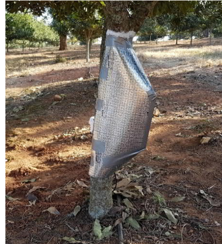
Protected sap-flow sensor on a macadamia tree.
