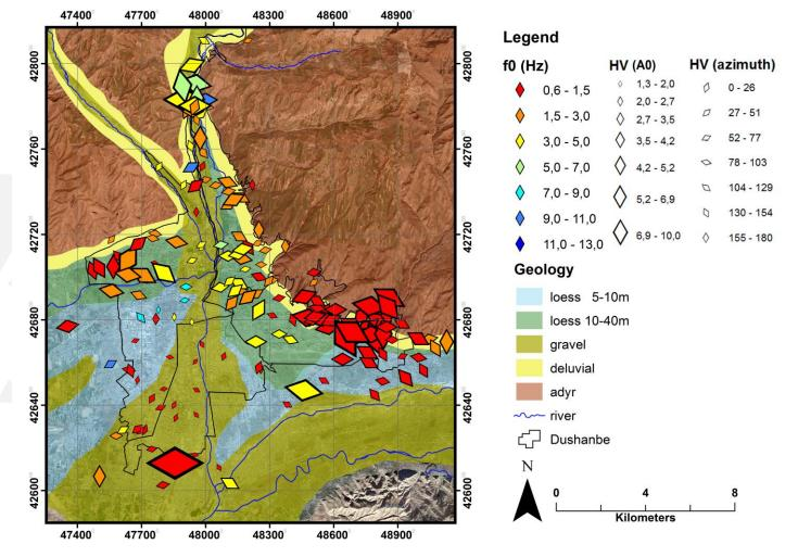
Passive – source recording of ambient noise: HVSR
