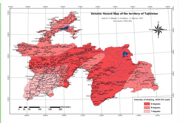
Based on the geological and seismological data the general seismic zoning map in terms of intensity by MSK-64 scale of the territory of Tajikistan was created in 1978 (Babaev et. al, 1978), and it uses as the seismic building code till now.
