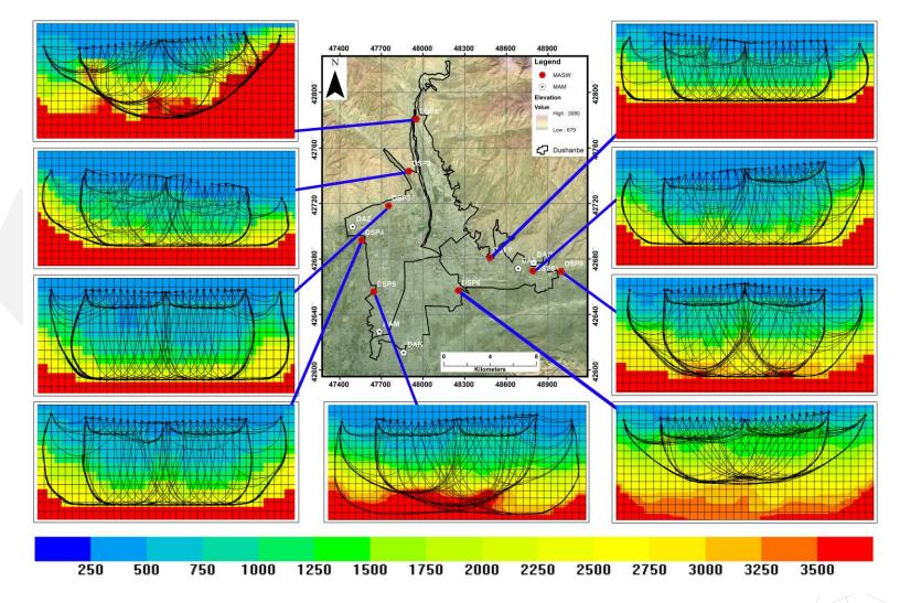
Passive – source recording of ambient noise: HVSR
