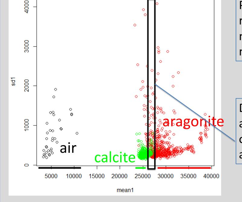
radiodensity for each reference material and air to identify reliable min-max radiodensity boundaries
