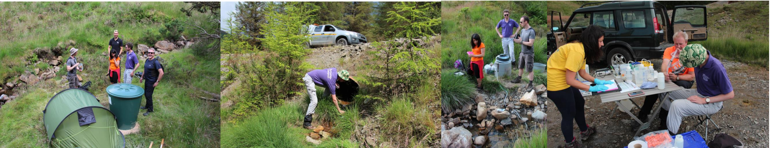
L-R: Sodium Bromide tank and injection site; collecting samples; one of three autosamplers; field laboratory filtering and fixing samples for future analysis (Edwards 2019)
