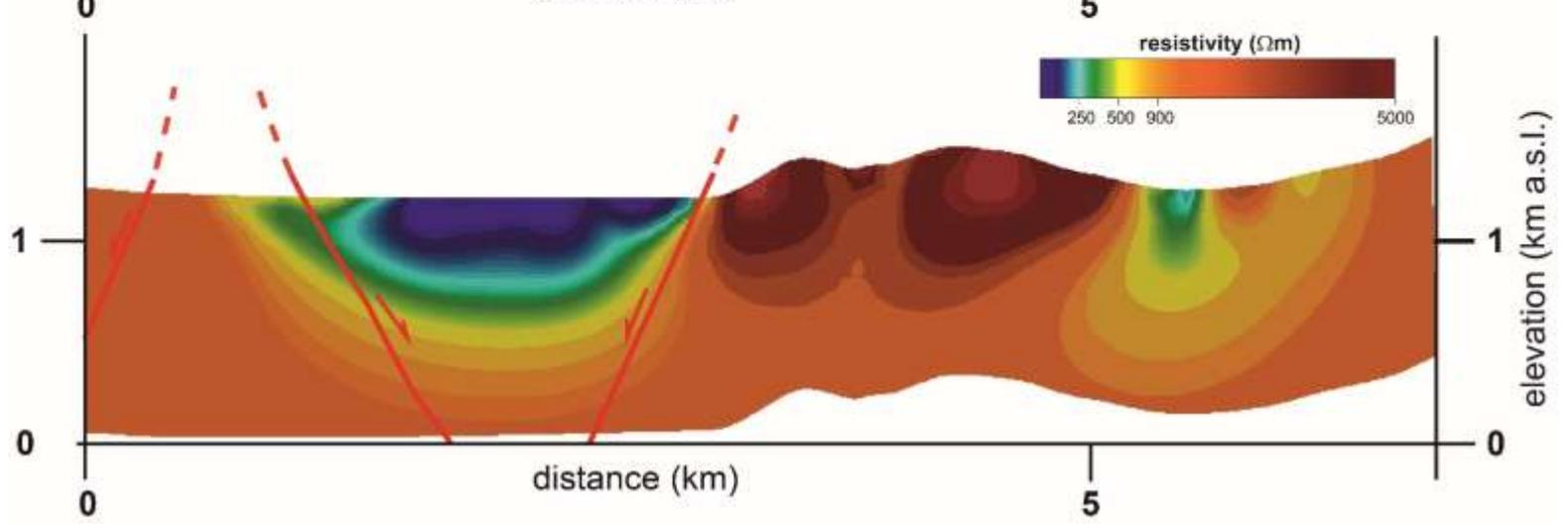
Sketch of **possible deep fault networks** as inferred from the recovered 3D resistivity model (elevation slice at 900 m a.s.l.).
