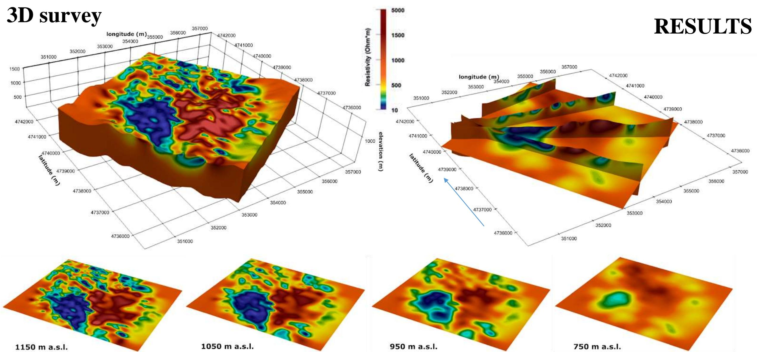
**Top left:** 3-D Fullwaver resistivity model of the entire survey area. **Top right:** 2-D cross-sections over the horizontal slice at 750 m a.s.l. **Bottom:** slices at different absolute elevations. The wide low-resistive region delineates the deeper portion of the PGC basin infill. Those slices suggest a complex structure with a main depocenter to the south and segmentation to the north, due to the interference of differently oriented fault systems
