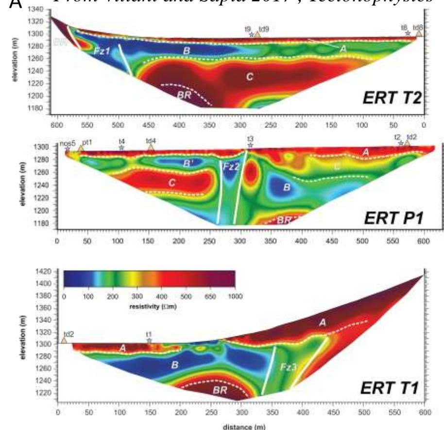
A - The dashed lines indicate approximate boundaries of the main electrical units: A and C: alluvial fan deposits; B: fluvio-lacustrine deposits; BR: carbonate bedrock. The lateral extent of the inferred fault zones (**units Fz**) is shown with solid white lines.
