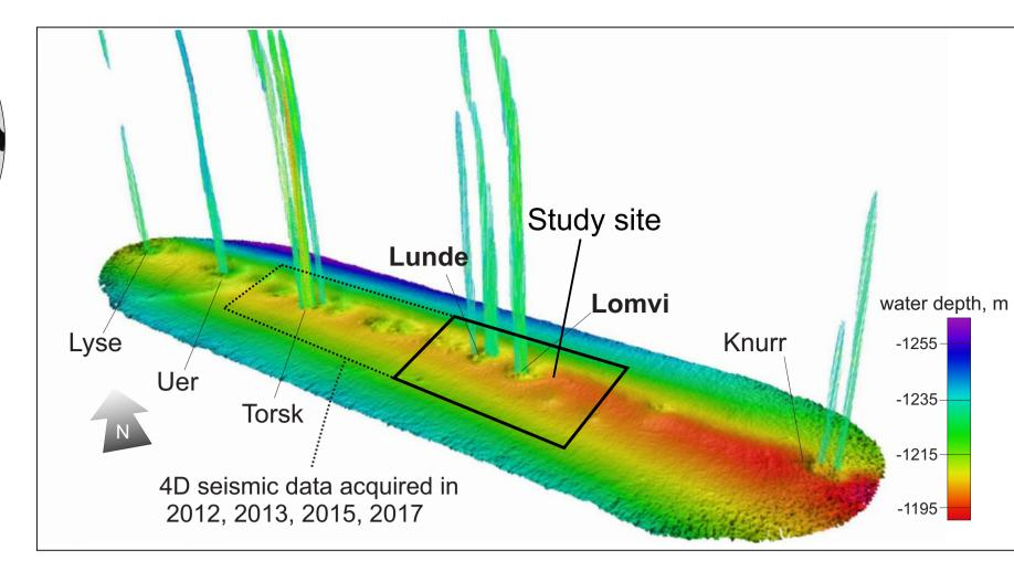
800 m - tall echosounder signals capturing gas bubbles in the water column.
