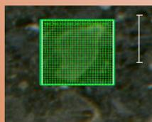
**Fig 3:** A 30 X 30 grid was placed over a shard and XPS analysis was conducted in each cell. Scale bar = 1 mm
