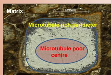
**Fig 2:** A Basaltic glass shard showing zone where the morphological biosignature can be observed. Scale bar = 100 µm
