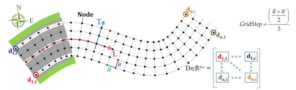
The elevation value of each single node of the two-dimensional grid is estimated by means of spatial interpolation processes
