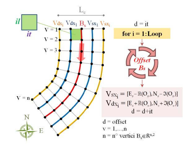
Repeated sequences of instructions generate numerous variables with the same names; for this reasons all outputs are organized in Structure Array. In particular, the planimetric coordinates of the nodes are organized in Multidimensional Arrays  $D \in \mathbb{R}^{n,(2 \cdot Loop+1),2}$ , an extension of a twodimensional matrix.
