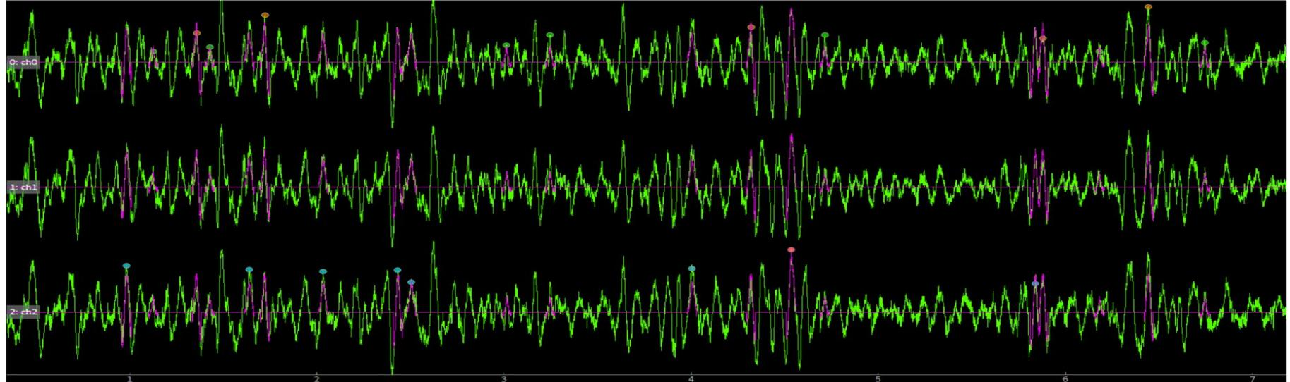
Waveform selection: on the basis of waveform template. Signals almost replicate with a small lag (300 ms lag).
