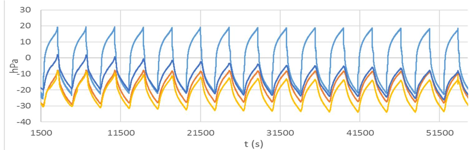
Pseudo-structure induced by injecting air bubbles led to a major occurrence of pressure jumps.
