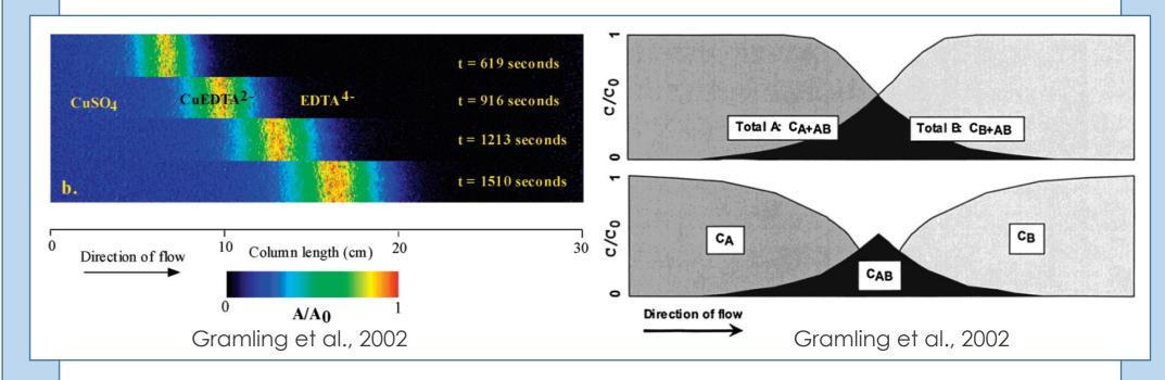
Gramling et al's 2002 experiment [5]: watersaturated sand through which two reactants mix by dispersion and react. Discrepancy btw. ADRE prediction & observations. Results are reproduced with proposed approach:
