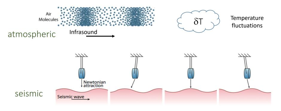
Gravitational coupling between the mirrors and surrounding mass density fluctuations
