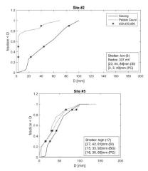
Figure 3: Results of the measurements of the grain size distribution using sieving, basegrain and pebble count at two different spots in the part-time submerged (#5) and submerged (#2) region
