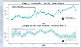
The oxygenation of subsurface water is closely related to the intensity of cold water formation. In 2017 and 2018,, a substantial amount of cold water was formed, which resulted in a partial reoxygenation of the intermediate layer and provided, at least, a temporary relief in the preceding deoxygenation trend.
