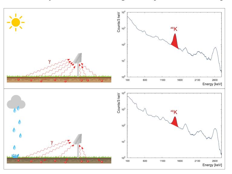
The **soil water content w** (M<sub>water</sub>/M<sub>soil</sub>) is **inversely proportional** to the signal **S(K)** produced by the <sup>40</sup>K decay measured by the gamma spectrometer:
