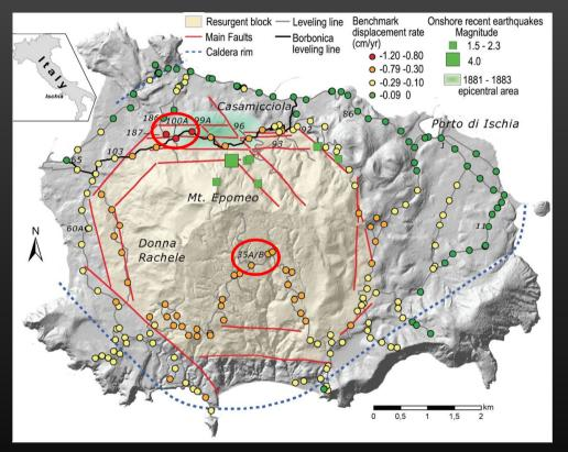
The self-similarity of the normalized patterns and the constant ratio between 35A and 100A benchmarks suggest the activity of the same source/s and interdependence in the process/es controlling the deformation at Ischia
