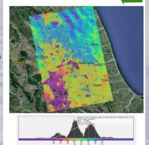
Snow depth Principle: variation proportional to SAR differential phase (known incidence angle, frequency and snow density) for each pixel
