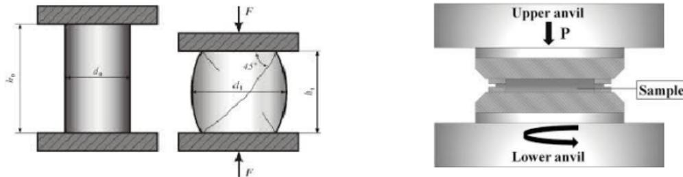
*Schemes of two experiments – on compression and on high pressure torsion*
