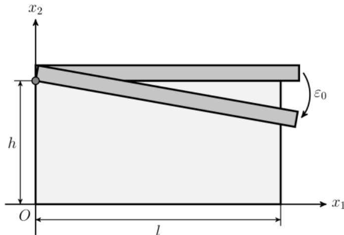
*Scheme of a medium loading by a rotating plate*
