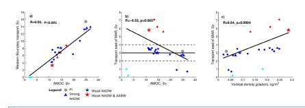
(a) As the AMOC weakens, so does the deep western boundary current (b) However, the mid-depth southward transport on the east side of the Mid-Atlantic Ridge (MAR) strengthen as the AMOC weakens and NADW becomes shallo (c) This strengthening on the east side of the MAR is associated with an increase in vertical density gradient (b) However, the mid-depth south (c) This strengthening on the east
