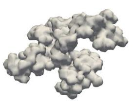
number of monomers N=26-1508 fractal dimension  $D_f=2.2$ (describes compactness, for sphere  $D_f=3$ ) fractal prefactor **k**<sub>0</sub>=1.625 (describes packing density along branch, the higher  $k_0$  the denser the packing) monomer radius a=28 nm overlap factor C<sub>ov</sub>=0.33 (quantifies overlap between monomers,  $C_{ov}=0$  point-contact,  $C_{ov}=1$ , full overlap)
