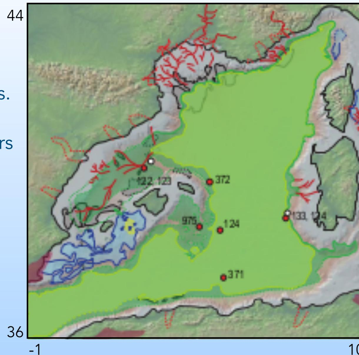
Detail from extension map of the MSC seismic markers in the Western Mediterranean, showing Mobile Unit (yellow), Upper Unit (green), and Complex Unit (blue) distributions, from: *Seismic Atlas of the Messinian Salinity Crisis markers in the Mediterranean Sea - Volume 2* (Lofi et al., 2018)
