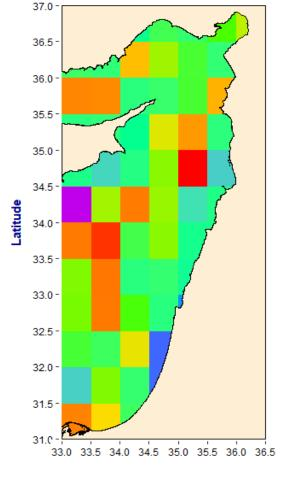
Difference between DTU18MSS & Gauss-Markov (cm)
