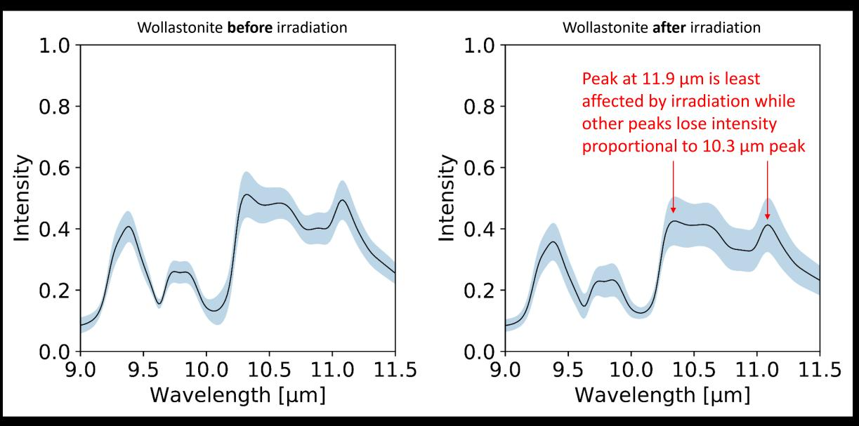
Note: range was chosen to highlight extrema; black line = mean over 10 measurements; blue area = 2SD.
