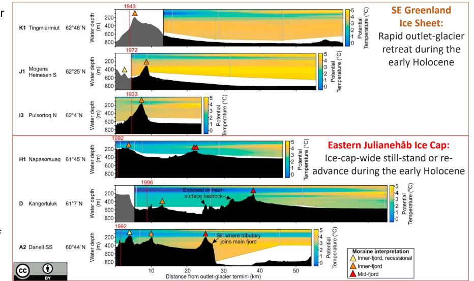
**Fig. 4.** Selected profiles along the fjords of SE Greenland, showing the locations of major moraines and the potential water temperature of the fjords. The black and grey areas show seafloor depth from OMG bathymetric data and free-air gravity anomaly data, respectively. Dashed red lines are former outlet-glacier positions. Adapted from Batchelor *et al.* (2019).
