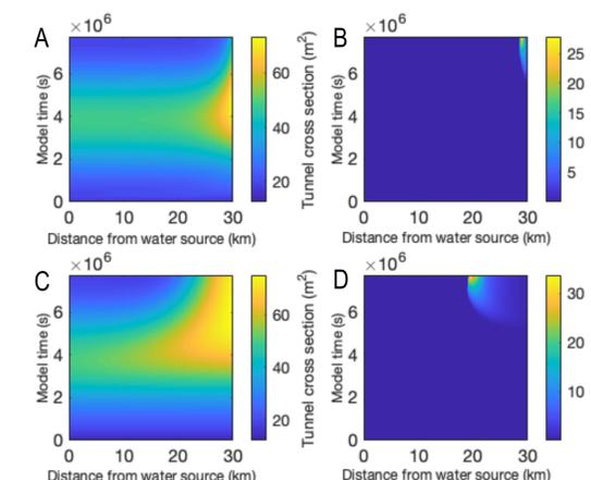
Figure 4. Time/space diagrams for evolution of tunnel cross section and sediment thickness. Discharge forcing is symmetric through time; peak discharge of  $200 \text{ m}^3 \text{ s}^{-1}$  is half way through run. A: Earth  $g$ , tunnel cross section. B: Earth  $g$ , sediment thickness. C: Mars  $g$ , tunnel cross section. D: Mars  $g$ , sediment thickness.  $\rho_w = 1000 \text{ kg m}^{-3}$ ,  $A = 5 \times 10^{-26} \text{ Pa}^{-3} \text{ s}^{-1}$
