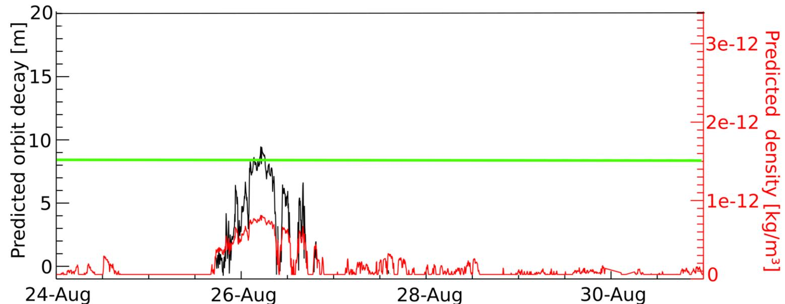
Predicted orbit decay (black line) and thermospheric density (red line) for a fixed altitude of 490 km. The green line indicates the post-processed maximum orbit decay for the GRACE-C satellite during the storm period in August 2018.
