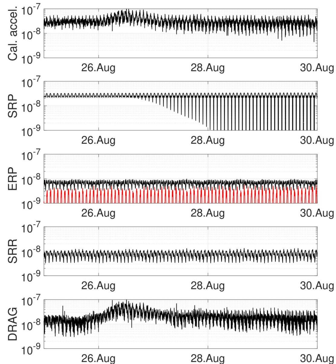
Calibrated accelerations of GRACE-C (units are  $\text{ms}^{-2}$ ), accelerations due to SRP, ERP (visible (red) and infrared range (black)), SRR and the final estimated non-gravitational accelerations due to atmospheric drag.
