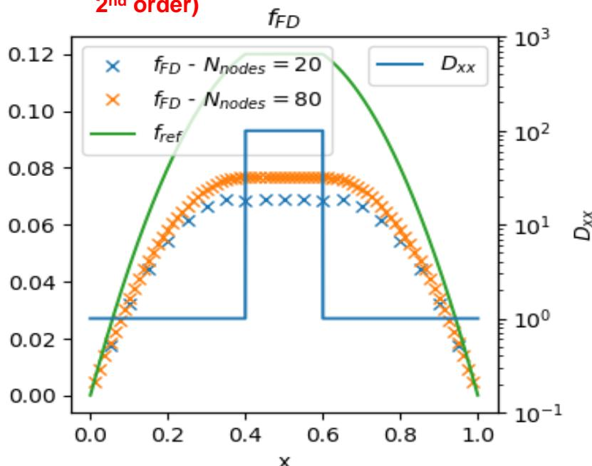
FD test on unidimensional stationary diffusion with discontinuous coefficient
