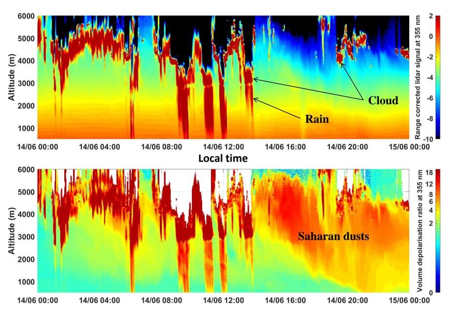
The spatio-temporal location of aerosols by lidar makes it possible to identify the presence of air masses of potentially different origins and therefore with a different moisture history.
