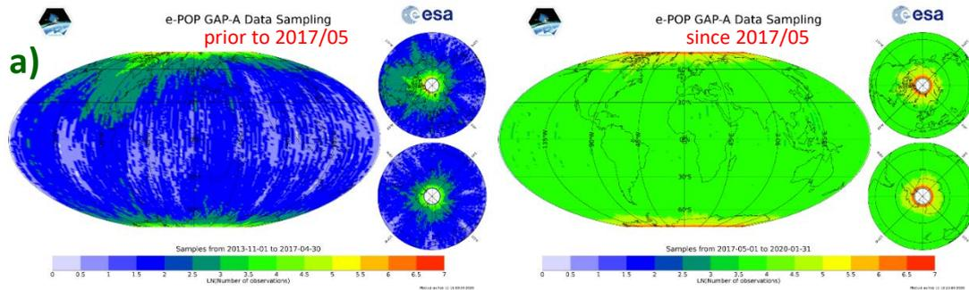
Full-orbit GAP-A data (1-20 Hz) are required to yield spacecraft positions of sub-decimeter RMS uncertainty and to derive *localized* spacecraft acceleration (or deceleration)
