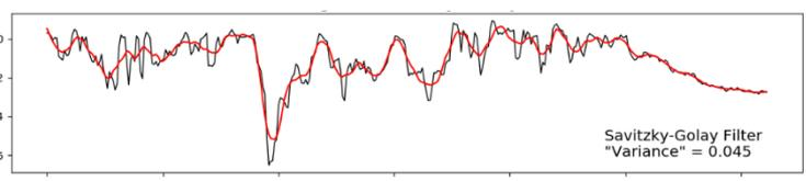
IRM measures incident plasma current at  $10^3$  samples/s, and uses data to infer small-scale (10-100 m) density structure ( $n_e$ ,  $\Delta n_e/n_e$ )
