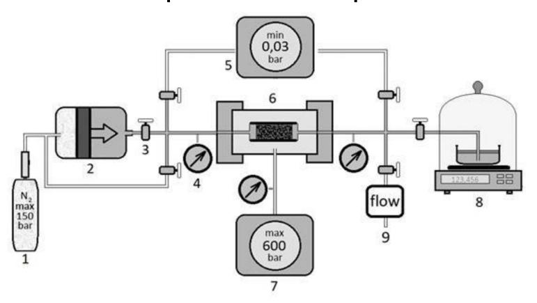
Fig. I. Experimental setup. I – buffer tank; 2 – hydroaccumulator; 3 – valves; 4 – pressure sensors; 5 – vacuum pump; 6 – core holder; 7 – high pressure pump; 8 – balance with tank for accumulated fluid; 9 – thermal mass flow meter
