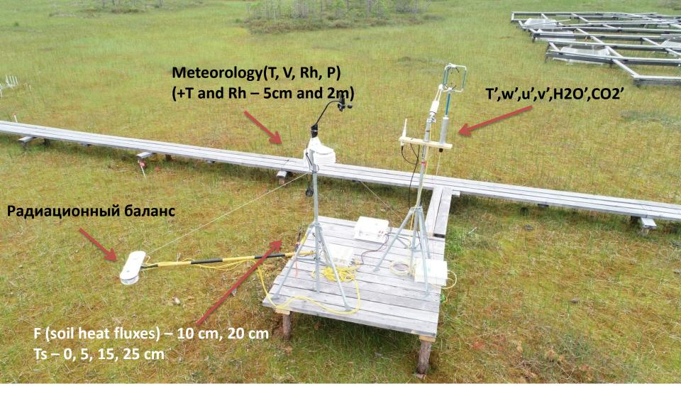
Turbulent fluxes of momentum, sensible and latent heat, and CO2 were measured with the EC technique. Measurements in the atmosphere were supplemented by measurements of heat flux through the soil, radiation balance and soil temperature at several levels. Surface
