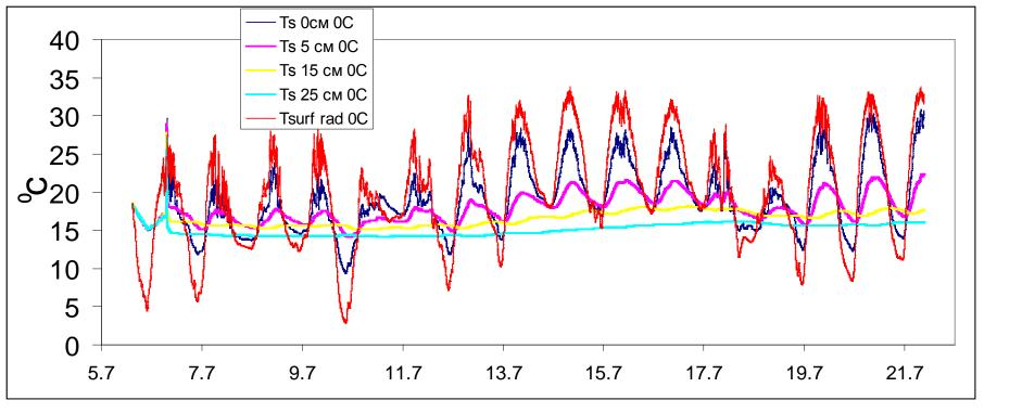
The daily temperature variation practically disappeared at a depth of 15 cm. A significant difference was observed between the surface temperature measured by a radiometer and a contact sensor, which indicates the existence of a skin layer.
