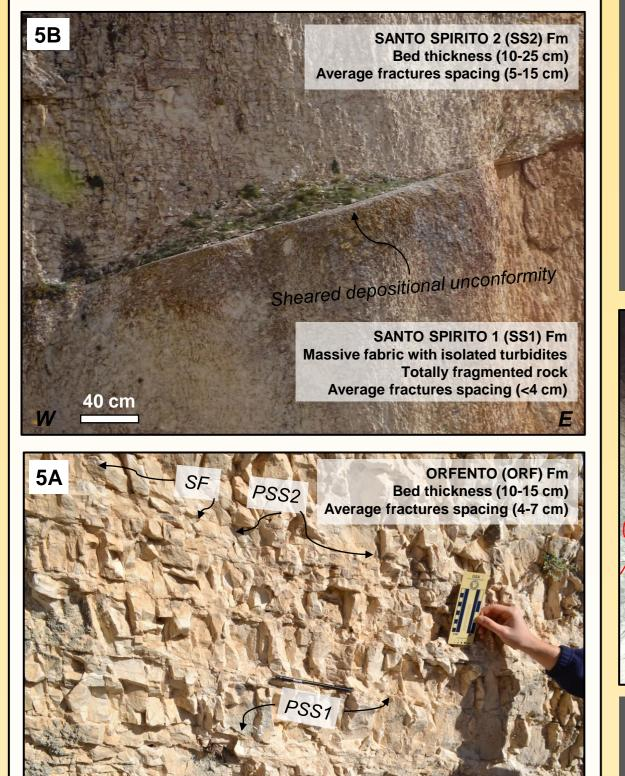
◀ Fig. 5 – Background structural assemblages in Orfento Fm (A) and Santo Spirito Fm (B). Background deformation structures (J1, J2 and PSS2) are mainly strata bound and just occasionally through-going. Obliqueangle splay fractures (SF) on sheared PSS1 and bedding interfaces are present both in ORF Fm and SS2 Fm. SS1 Fm is observed completely fragmented with fractures spacing generally < 4 cm.
