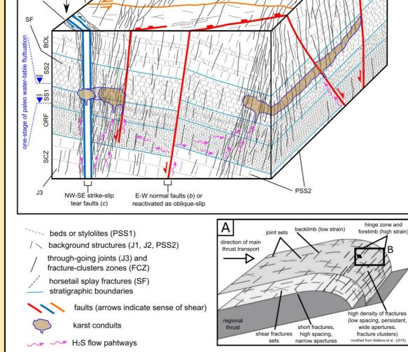
A) regional context in the thrust sheet; B) box diagram with surveyed structures in Taranta Valley and spatial distribution of karst conduits. H<sub>2</sub>S-bearing fluids came from deepburied Triassic evaporites at the base of the thrust.
