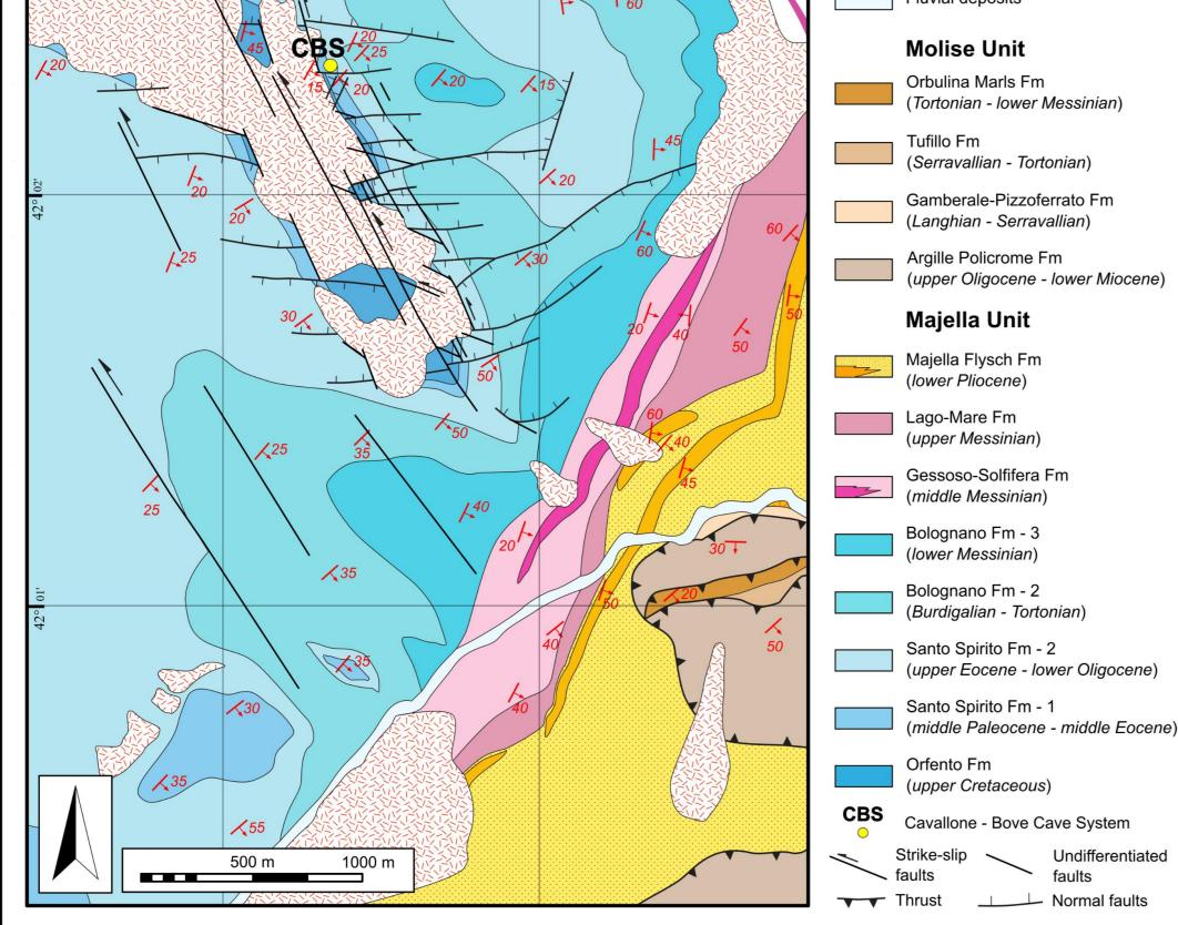
▲ Fig. 3 – New geologic map of the Taranta Valley, in Majella Massif, with the main structures observed (modified from Festa et al., 2014).
