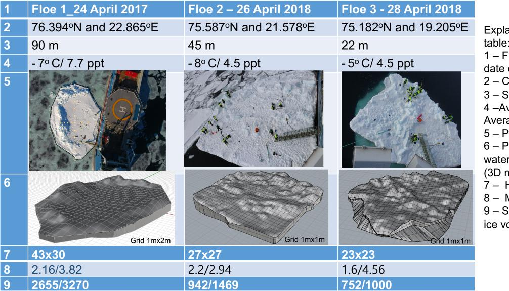
Explanation of the lines in the table: 1 – Floe number and date of observation. 2 – Coordinates, 3 - Sea depth in the place,4 – Average Air Temperature / Average Ice Salinity, 5 – Photo, 6 – Perspective view of above water surface and side wall (3D model), 7 – Horizontal size, m., 8 – Max Sail/ Draft, m., 9 – Submerged volume/Total ice volume, m<sup>3</sup>
