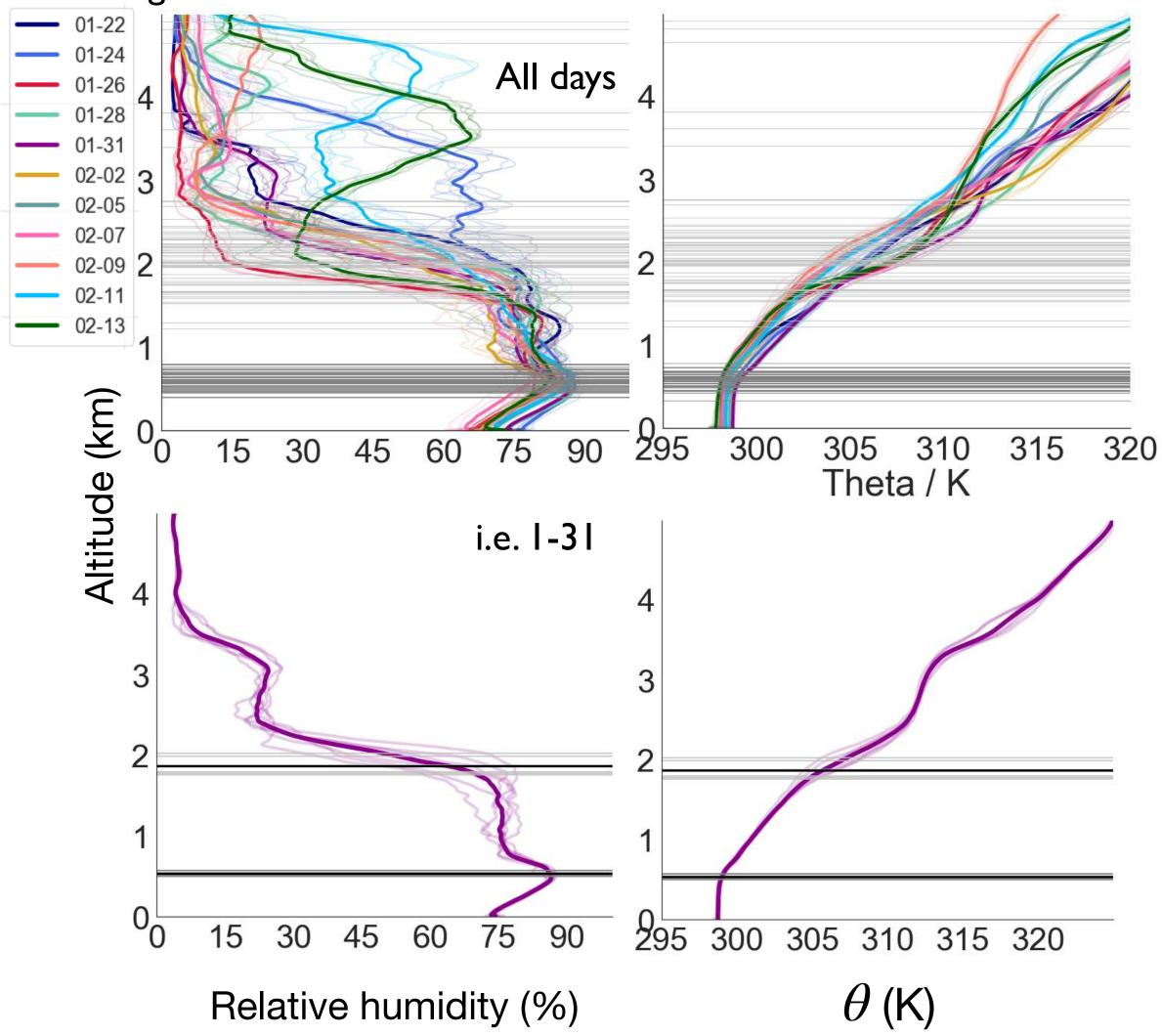
Mixed layer height from RHmax or  $\partial \theta / \partial z$  denoted by grey lines; inversion base height from where static stability first exceeds 0.1K/hPa given by silver lines. For I-31, black line corresponds to flight-mean mixed layer or inversion base height.
