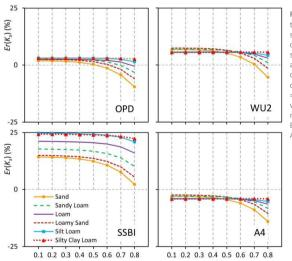
Figure 3. Relative error of the estimated values for saturated soil hydraulic conductivity, Er(Ks), for six synthetic soils that were analyzed using four different methods. OPD = one-ponding depth; WU2 = Method 2; SSBI = Steady version of the Simplified method based on a Beerkan Infiltration run; A4 = Approach 4.
