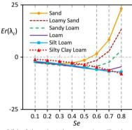
Figure 2. Relative error,  $Er(\lambda_c)$ , of the estimated macroscopic capillary length compared to reference values for six synthetic soils.
