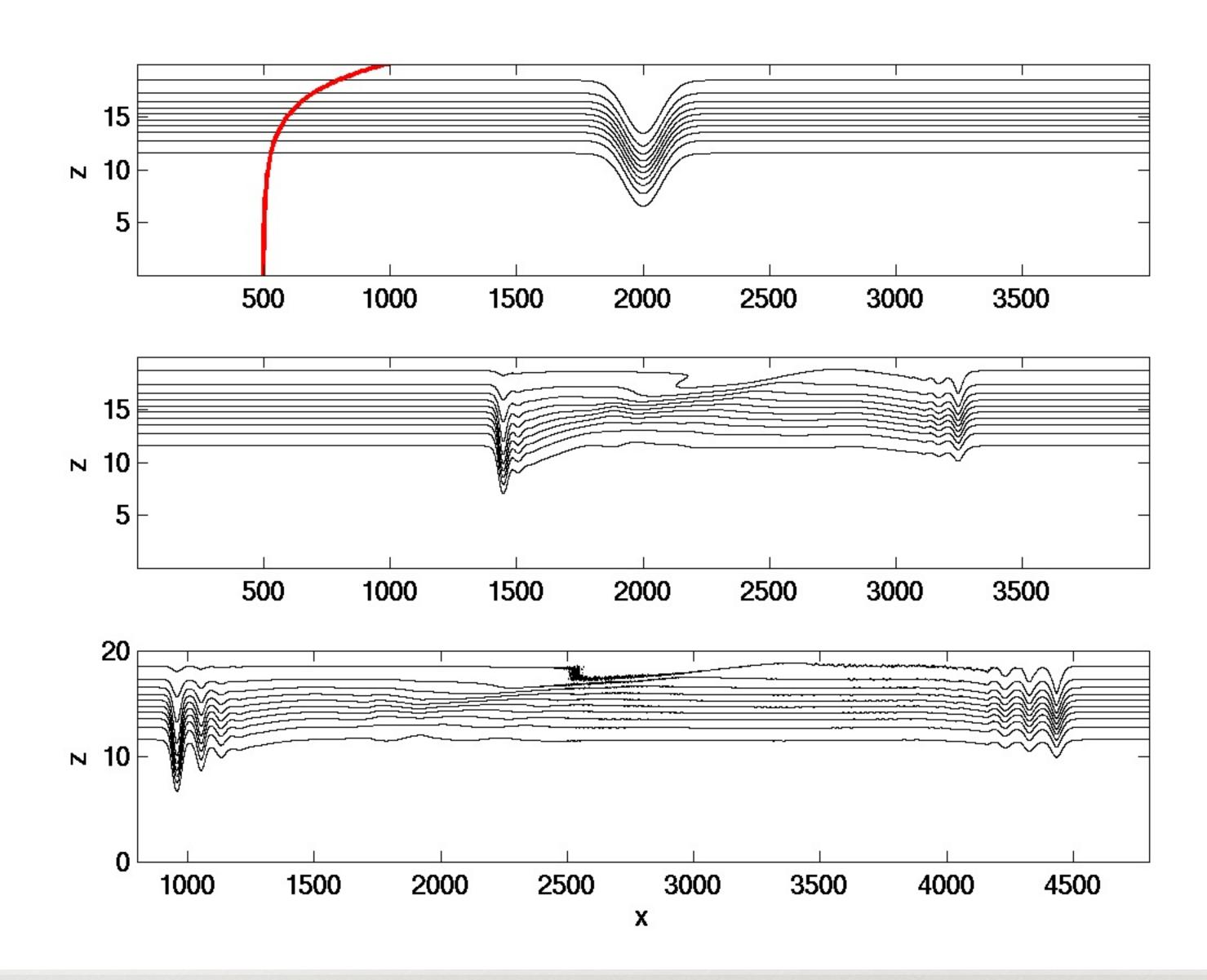
Strongest Current: Again coherent ISW trains but tail appears attached to rightward propagating waves. Short length scale shear instability observed
