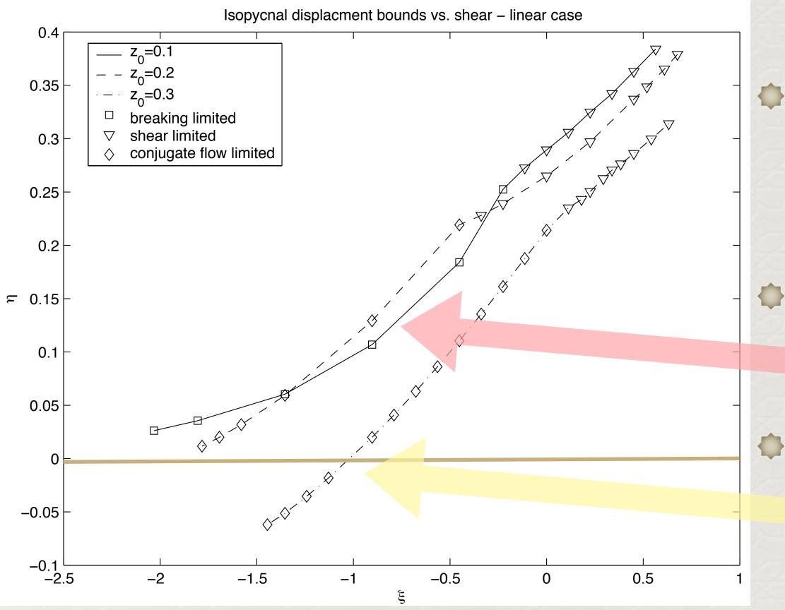
Fully nonlinear ISWs can be solved for up to some limiting amplitude
