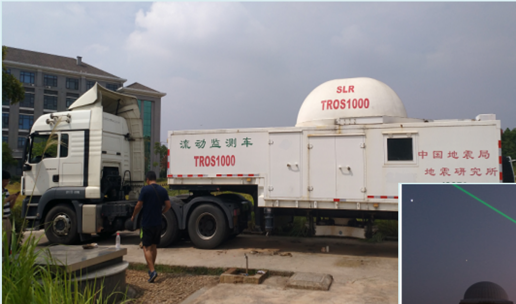
The mobile SLR system (TROS) in Xinjiang Observatory (Urumqi)
