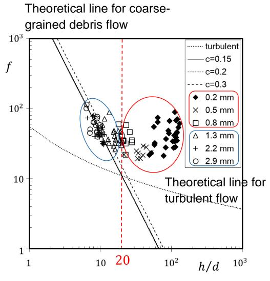
Theoretical friction coefficient for coarse-grained debris flow derived from constitutive eqs.
