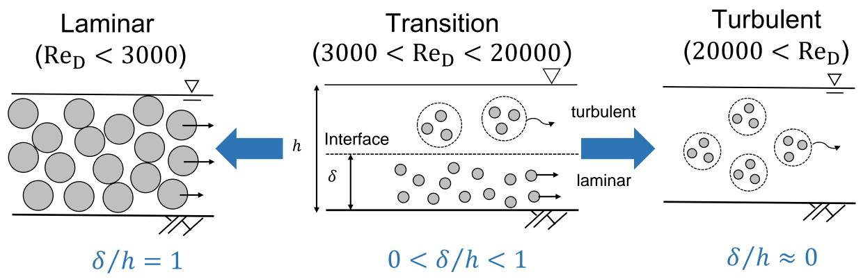
The laminar-turbulent transition in debris flow may be described in a unified view, using a two-layered model in which the position of the between-layer interface is varied depending on  $Re_D$
